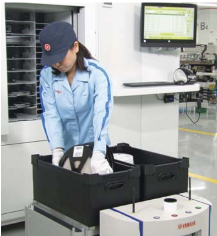
Photo 1: Delivery of components from the SMD storage system and transfer using AGV
