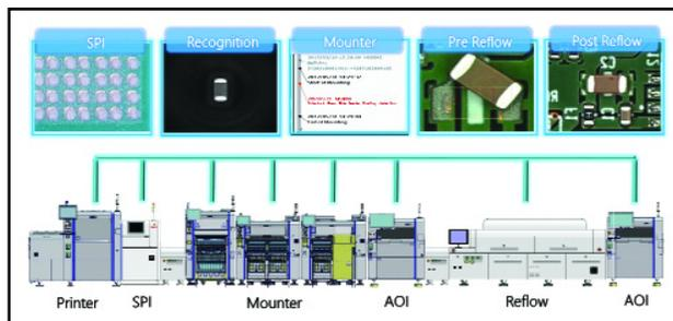
**SMT line with closed-loop feedback of SPI data to printer, AOI data to the moulder and the correlation of all data with traceability software.**
